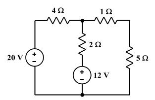
a. How many equations are necessary to analyze this circuit by the mesh analysis method?
